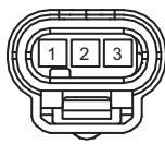
(B-017) B Low Pressure Fuel Pressure Sensor
